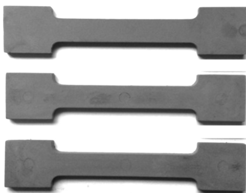
FIGURE 5. Parts injected at optimized injection molding parameters
